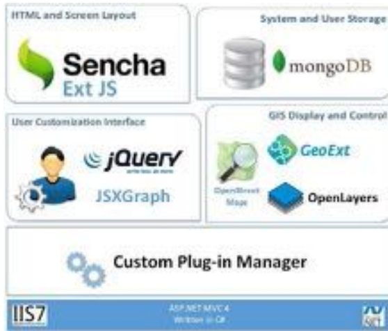
Figure 4. Framework for PVMapper Architecture.
